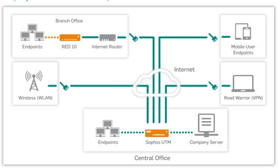
You can easily extend UTM protection to remote offices, mobile devices, WLANs and road warriors.
